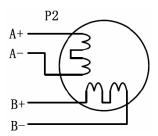
Figure 4: 4-lead Motor Connections
