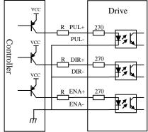
Figure 2 Connections to open-collector signal
