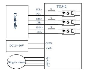
Figure 9 TD542 Typical connection
