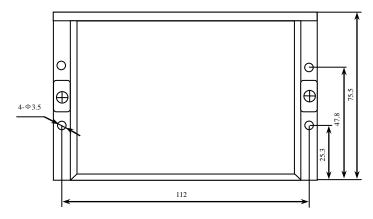
Figure 1: Mechanical specifications
