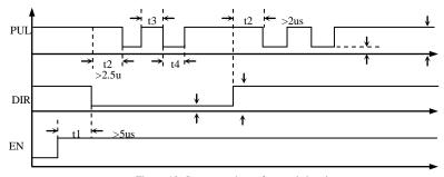
Figure 10: Sequence chart of control signals
