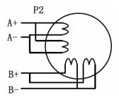
Figure 8: 8-lead motor parallel connections
